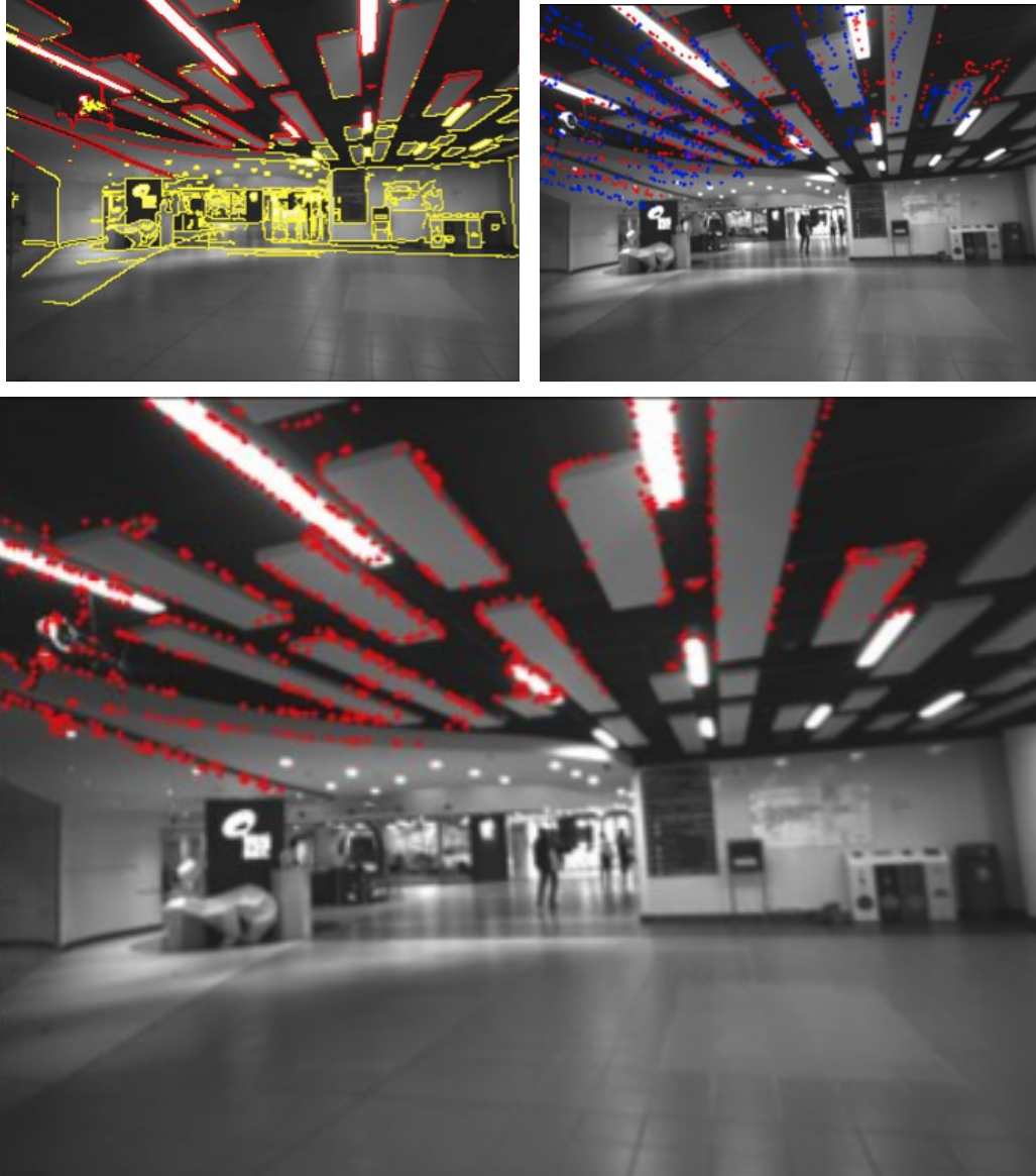
Figure 5.16: Top-row left: Detected edge-points marked on the current image. In yellow are all detected points. In red are the points with valid depths, ie. {}^cX . Top-row right: Reprojected edge-points of current image plotted on the reference image. In blue is the reprojection using pose computed with PNP(+RanSAC) on ORB sparse-point matches. In red is the reprojection using pose computed with PNP (+RanSAC) on matches with GMS-Matcher [18], ie. {}^rT_c^{(PNP)} \times {}^cX . Bottom: Reprojection of detected edge points of current image plotted in reference image using pose computed by proposed edge-alignment method, {}^rT_c^{(EA)} \times {}^cX .
