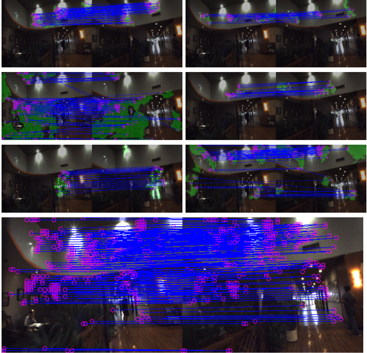
Figure 5.3: 23 consistent matches with sparse features. 312 matches with proposed method. The green overlays are the clusters with same index from association map.
